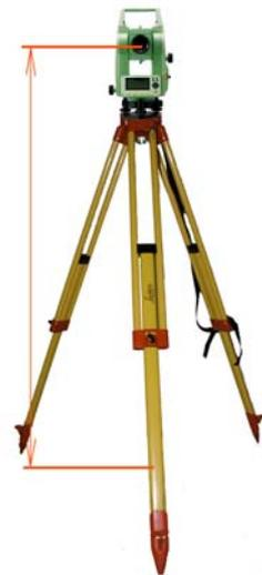
**6.** With the plummet centred on the point the instrument is now levelled by adjustment of the tripod legs. Working on each leg in turn slacken off the clamping screw and slide the leg to bring the instrument bubble in line with its centre circle. Re-tighten the clamping screw securely before adjusting the next.
