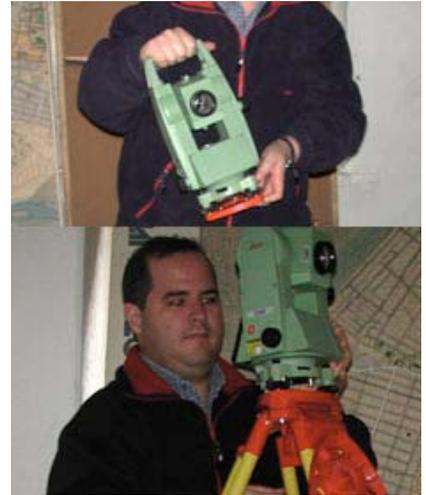
**3.** Place the instrument carefully on the tripod. Check the tripod is stable, the stage roughly level and the plummet is over the point.
