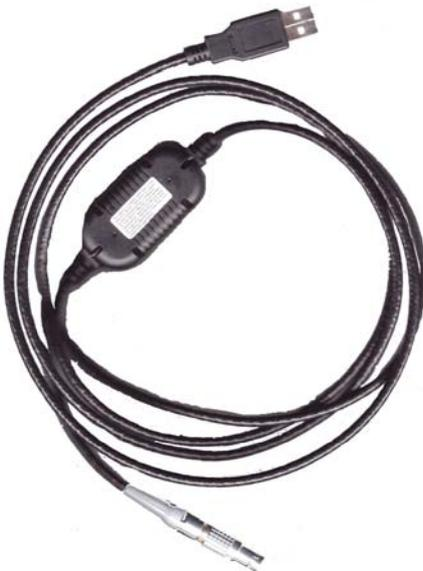
**5.3. Leica GEV 189 USB serial cable:** this cable can be used as a replacement for the standard Dsub 9 cable. It is supplied with the required drivers and works in much the same way as the USB to serial adapter but with the advantage of being a single piece. The cable is less stable than its serial predecessor and cannot be disconnected from the PC without terminating the TheoLt session.
