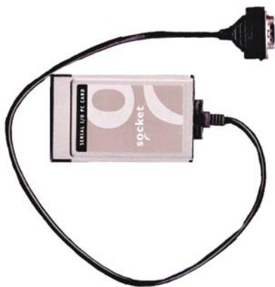
**5.1 PCMCIA serial adapter:** fits in the PCMCIA port on the computer and allows the standard communication cable to be used. This is the most stable option as the card uses long standing drivers and can recover from accidental removal during use. It will need installing with the correct drivers and the port assignment can be identified by using the *un-plug or eject hardware* icon in the system tray.
