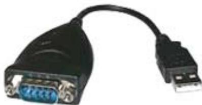
**5.2. USB to serial adapter:** these devices tend to pull on the USB port on the PC and unplug themselves easily: this is unwelcome because the drivers for them cannot cope with make and break connection. Cheaper than the PCMCIA option but risky.
