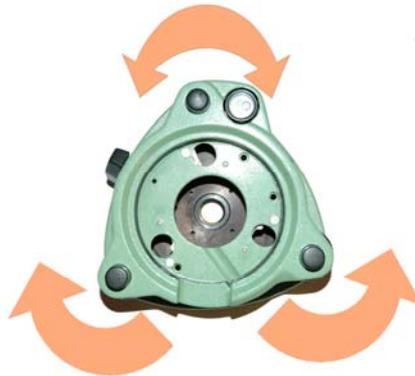
**5.** Once close to the point fine adjustment is done with the tribrach foot-screws. Use 2 of the foot screws by turning your thumbs out or in together [but never turning them in the same direction] to move the plummet onto the point. The 3<sup>rd</sup> screw will provide the motion to move at right angles to the first movement.
