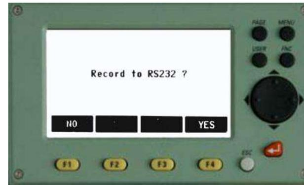
Note that the first shot taken with the All key will prompt a 'Record to RS232?' message on the instrument which should be confirmed with a Yes (F4) response.
